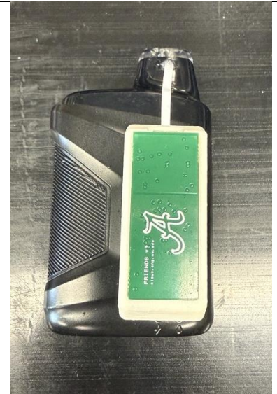
Figure 18. Vape with FRIENDS Device & thermistor installed
