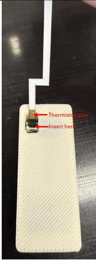
Figure 6. Proper orientation for thermistor cord installation
