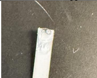
Figure 4. Thermistor with silicone applied (top view)
