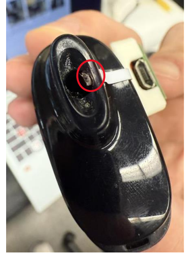
Figure 15. View of thermistor inside mouthpiece after installation
