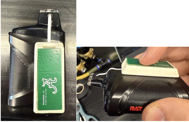
Figure 14. FRIENDS Device installed on vape
