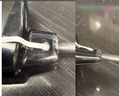
Figure 17. Thermistor hole sealed with dental bead
