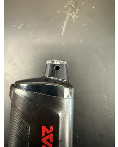
Figure 13. Thermistor hole on mouthpiece after drilling
