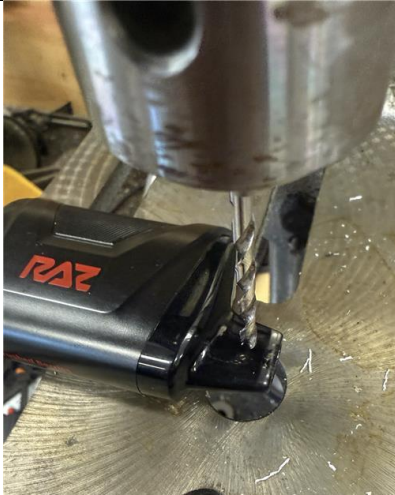
Figure 11. Determine vape position on platform using powered-off drill press
