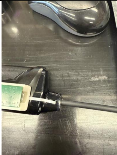
Figure 16. Vape with tubing inserted into mouthpiece for sealant application
