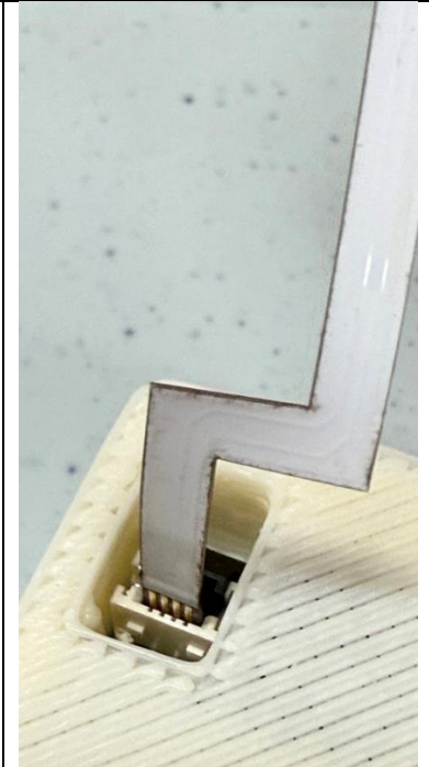
Figure 8. Thermistor cord properly inserted into FRIENDS device
