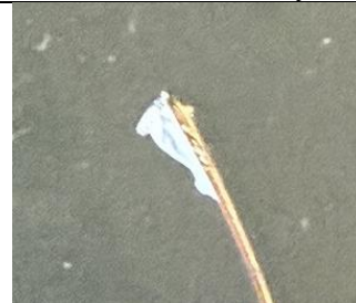
Figure 5. Thermistor with silicone applied (side view)
